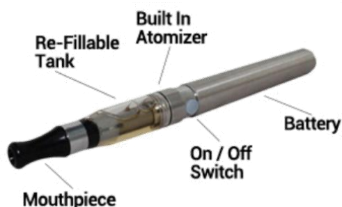
Figure 1 Main components of an e-cigarette
